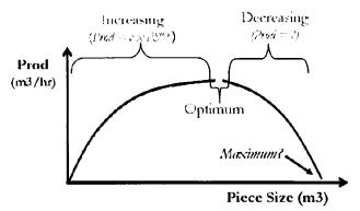
The productivity of any specific phase of a log harvesting operation is typically optimized to the design capability of the machine employed to conduct that phase. As can be seen above, as the piece size becomes smaller, productivity of machines (and logging phases) declines and costs rise. The same is true when piece size exceeds the optimum design capability of the machine in question. In this case, productivity also declines and costs rise.
