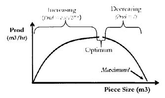
The productivity of any specific phase of a log harvesting operation is typically optimized to the design capability of the machine employed to conduct that phase. As can be seen above, as the piece size becomes smaller, productivity of machines (and logging phases) declines and costs rise. The same is true when piece size exceeds the optimum design capability of the machine in question. In this case, productivity also declines and costs rise.
