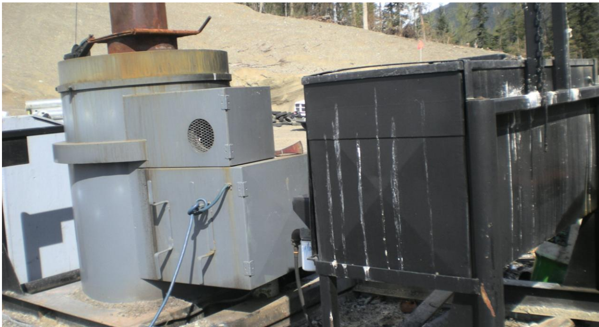
ECO Burn - Incinerator
