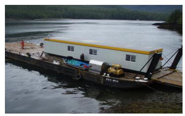
Hull Identification Number:179088 Home Port: Vancouver, British Columbia Tonnage: 107.49 GRT Type of Vessel: Steel deck barge Year Built: 1946 / 2008 Builder: Yarrows Shipyard, Esquimalt, British Columbia Estimated Speed of Vessel: 8 -12 knots Length: 30.48 m Beam: 8.23 m Depth: 1.46 m Construction: All welded steel; nine (9) compartments and access hatches
